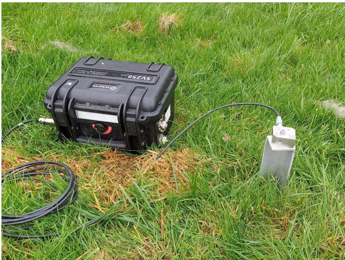
Figure 15: Photograph showing the vibration logging equipment used on a vibration spike at the northern façade location.
