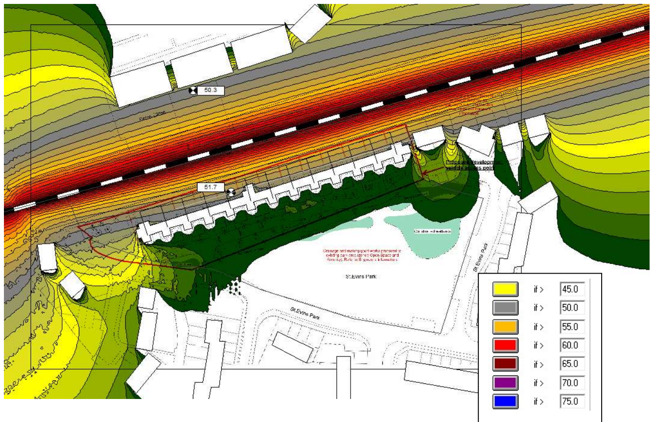
Figure 12: Showing a night noise contour map (LAeq,8hour) of the site for the night period at 1.6m above ground level proposed residential scheme at St Evins Park, Monasterevin, Co. Kildare.
